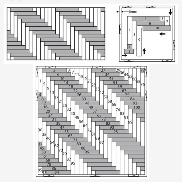
This sequence is given as an example, it will depend on the shape of the room. The important is to always start with the planks placed against the walls.
