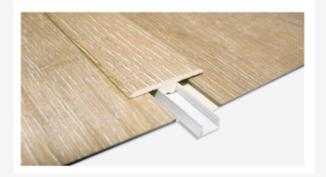
For surfaces over 400sqm, over 20m long or in the case of a surface where there has to be a transition from Click&Floor to a different floor tile, we recommend using T profiles taking care of the expansion joints (same joint that the perimeter joint)
