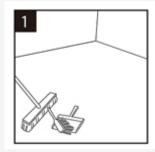
The subfloor should be even, dry, clean. Carpet staples or glue residues must be removed, and the floor must be clean to ensure proper installation.
