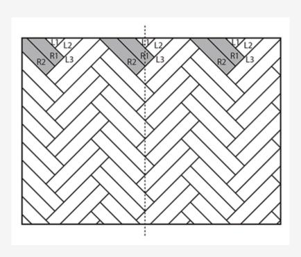
– For the double fishbone pattern, the cuts are different than what is indicated in the template inside of the box. Use measurements in below table to cut the 5 pieces (L1, L2, L3, R1, R2) of the starting set to the right size.
