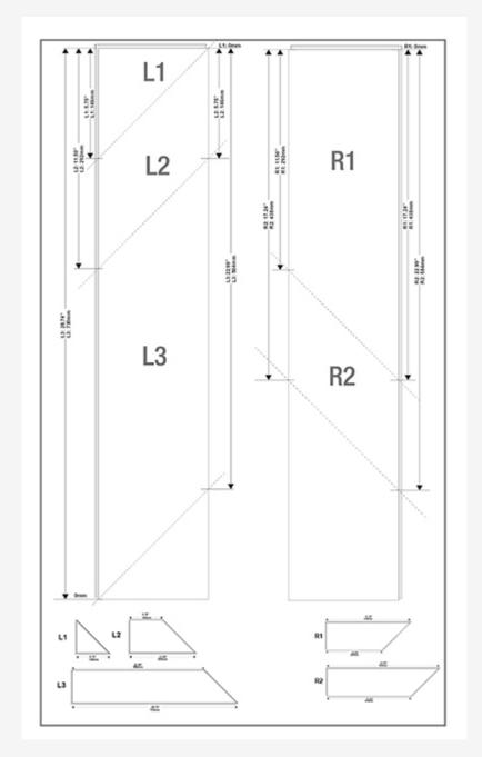
When you reach the walls on both sides, measure the distance between the wall and the closest starting set. Assemble a new set, mark the measured distance on it, cut the planks (the set can be disassembled for this) and install the planks in the gap.
