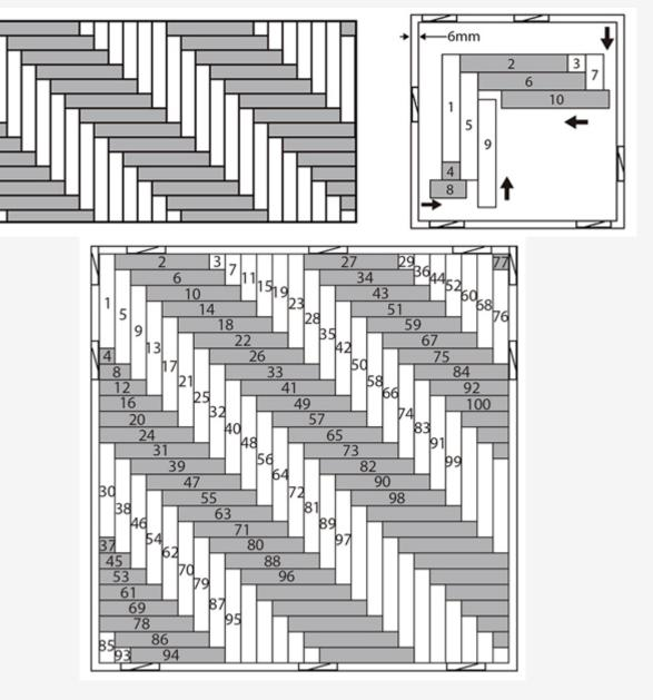
This sequence is given as an example, it will depend on the shape of the room. The important is to always start with the planks placed against the walls.
