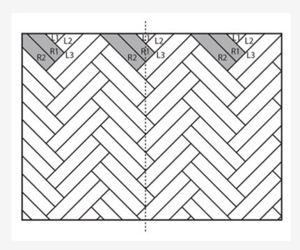
– For the double fishbone pattern, the cuts are different than what is indicated in the template inside of the box. Use measurements in below table to cut the 5 pieces (L1, L2, L3, R1, R2) of the starting set to the right size.
