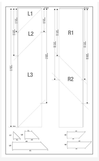
When you reach the walls on both sides, measure the distance between the wall and the closest starting set. Assemble a new set, mark the measured distance on it, cut the planks (the set can be disassembled for this) and install the planks in the gap.
