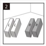
Separating into distinctive piles will make it easier to find the correct plank should the L or R markings be cut off.
