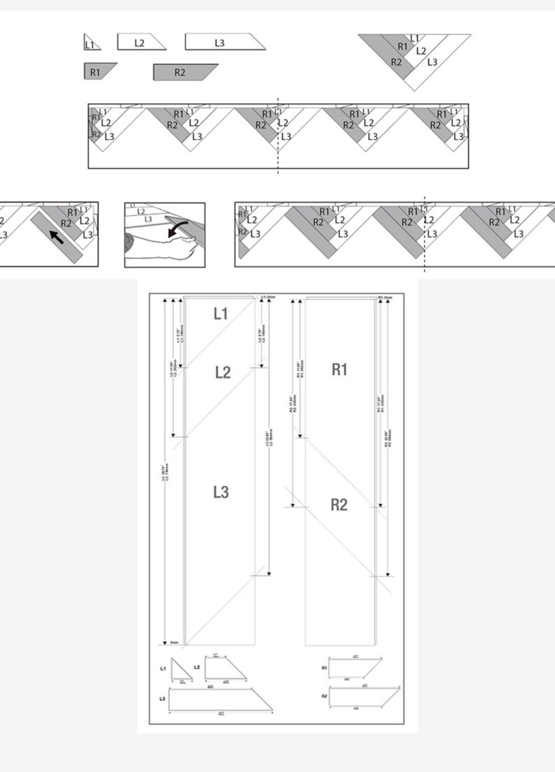
When you reach the walls on both sides, measure the distance between the wall and the closest starting set. Assemble a new set, mark the measured distance on it, cut the planks (the set can be disassembled for this) and install the planks in the gap.
