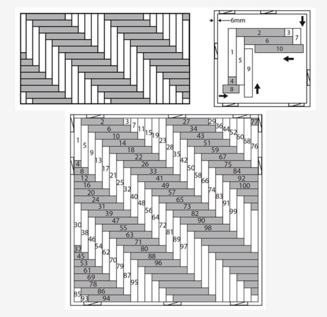
This sequence is given as an example, it will depend on the shape of the room. The important is to always start with the planks placed against the walls.
