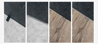
Lay the wall tiles at a height or 6 mm. Also place 10 mm perimeter gasket between wall and C&F. Fill the gap with silicone and place the board under the tile. Grout.
